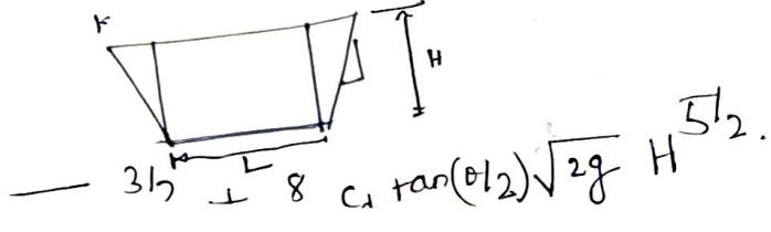
A right angled v-notch is inserted in the side of a tank of length 4m and width 2.5m. Initial height of water above the apex of the notch is 30cm. Find the height of water above apex if the time required to lower the head of tank from 30cm height is 3 minutes.  $C_d = 0.60$ .
