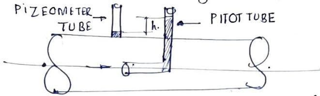
2. Pitot tube connected with piezometer tube:
