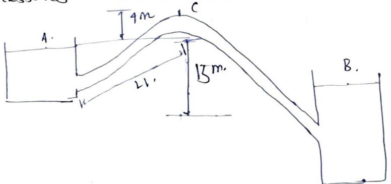
A Siphon of diameter 200mm connects two reservoirs having a difference in elevation of 20m. The length of the siphon is 500m and the summit is 3.0m above the water level in the upper reservoir. The length of the pipe from upper reservoir to summit is 100m. Determine the discharge through the siphon and also pressure at the summit. Neglect minor losses. The coefficient of friction  $f = 0.005$ .
