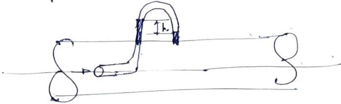
3. Pitot - Tube and Vertical Piezometer Tube, Connected with a differential manometer tube
