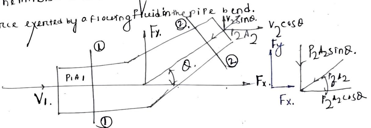
2. 250 Litres/second of water is flowing in a pipe having a diameter of 300 mm. If the pipe is bent by  $135^\circ$  (that is change from initial to final direction), Find the magnitude and direction of resultant force on the bend. The pressure of water flowing is  $39.24 \text{ N/cm}^2$ .
