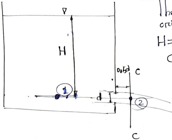
The tank is filled with a circular orifice.
