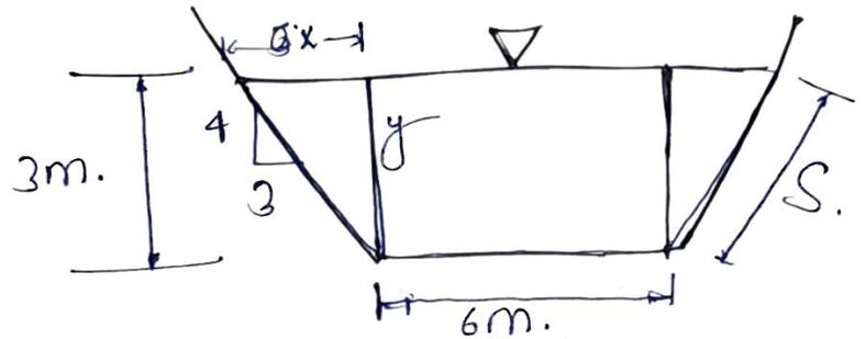
6. Find the discharge of water through the channel shown below. Take the value of chezy's constant  $c = 60$  and slope of the bed as  $1$  in  $2000$ .
