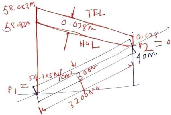
A pipeline 300mm in diameter and 3200m long is used to pump oil of density  $\rho = 950 \text{ kg/m}^3$  and whose kinematic viscosity is  $\nu = 2.1 \text{ Stokes}$ . The center of the pipeline at upper end is 40m above that at the lower end. The discharge at upper end is atmospheric. Find the pressure at the lower end and draw the HGL and TEL.
